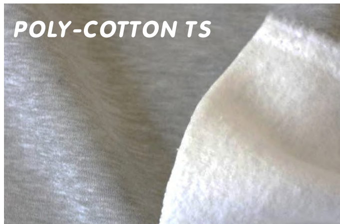
80% cotton, 20% polyester, grammage 270 g material from the inside finished with scratching (brushed)
