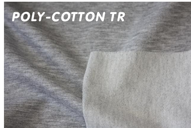
80% cotton, 20% polyester, grammage 270 g material from the inside finished with a loop
